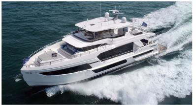
patented piercing bow and hull design, this latest FD75 is powered by twin Caterpillar C18 ACERTs of 1,136 bhp.
